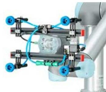
For instance, relative to Gimatic's new vacuum gripper product portfolio, the associated use of multistage vacuum pumps reduces energy consumption over traditional technologies thanks to intermittent on-off cycles, which enhances overall system efficiency.
